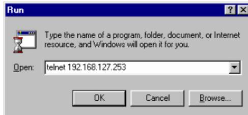
**NOTE** Telnet is not a default service in Windows 7 and later versions for a PC/laptop. In order to use the telnet service, you will need to activate it from **Control Panel** → **Programs** → **Turn Windows features on or off**. Select **Telnet Client** and press **OK**.
