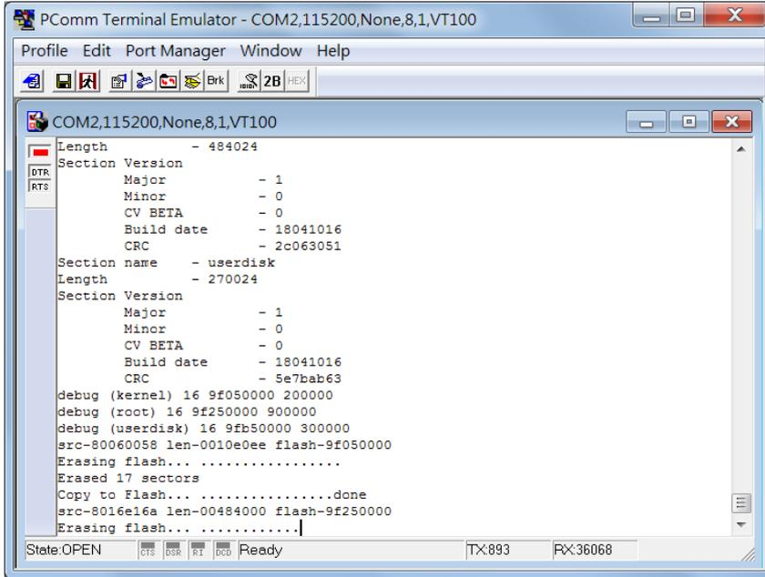
After the firmware recovering process is successfully completed, you will hear two short beeps and the STATE led on the device will turn green.
