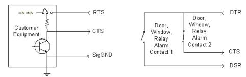
Figure 20 - Typical Alarm Inputs Connections
