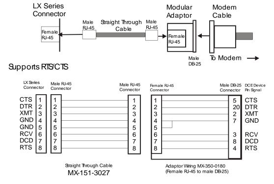
Figure 29 - Adapter Wiring, LX Series to DCE
