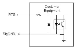
Figure 21 - Typical Interface Design for Control Output Signals
