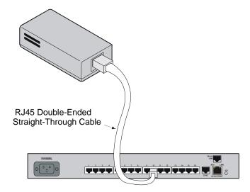
Figure 16 - Connecting the Temperature/Humidity Sensor
