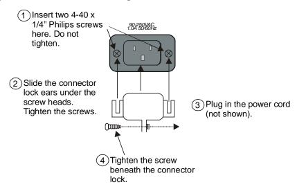
Figure 26 - Installing the Inlet Connector Lock
