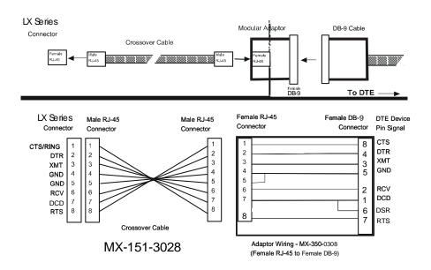
Figure 28 - Adapter Wiring, RJ-45 to DB-9, LX Series to DTE
