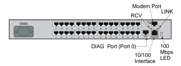
Figure 9 - LX Series 4032 with Modem Rear Panel
