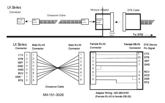
Figure 27 - Adapter Wiring, LX Series to DTE
