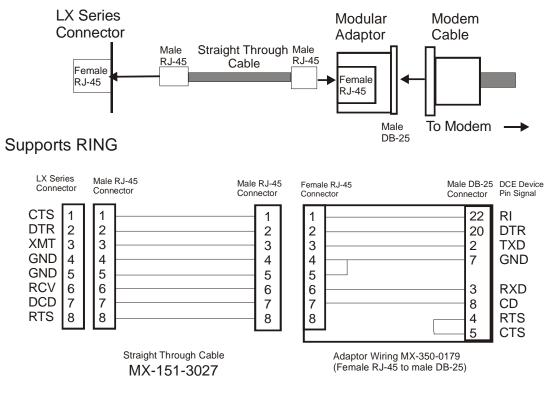
Figure 30 - Adapter Wiring, LX-Series to DCE, with RING
