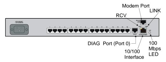
Figure 7 - LX Series 4016 with Modem Rear Panel
