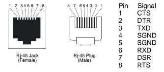
Figure 23 - Serial Device Connector (RJ-45) Signal Assignments
