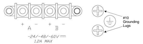
Figure 13 - Connecting DC Power
