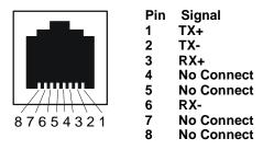
Figure 24 - 10/100 Connector Assignments
