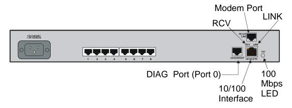
Figure 6 - LX Series 4008 with Modem Rear Panel
