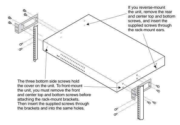
Figure 12 - Mounting an LX-4000 Series in Rack
