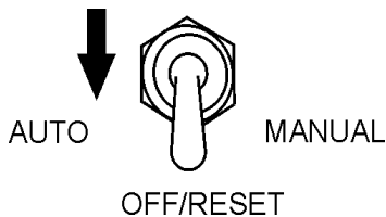
Figure 56. MPEC Control Switch (Off/Reset)
