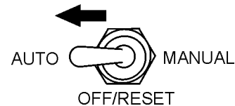
Figure 54. MPEC Control Switch (AUTO)
