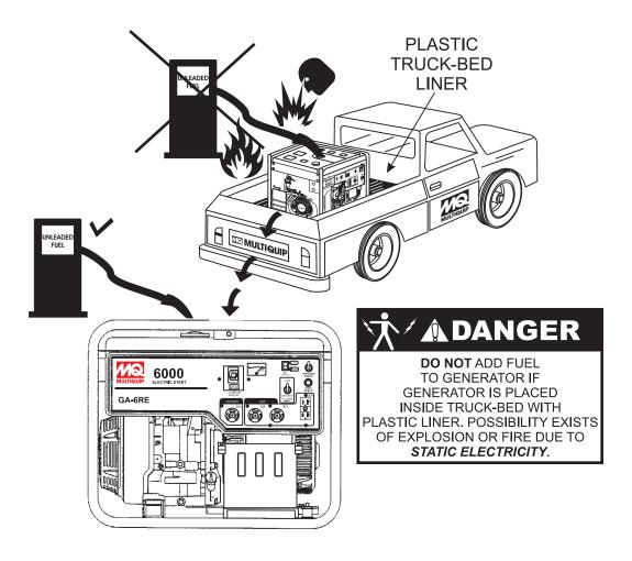
Figure 4. Generator Refueling
