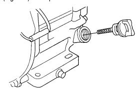
Figure 7. Engine Oil Dipstick (Removal)
