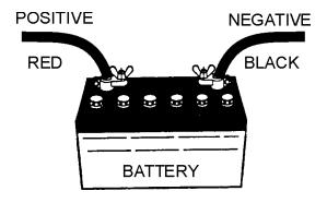
Figure 30. Battery Connections
