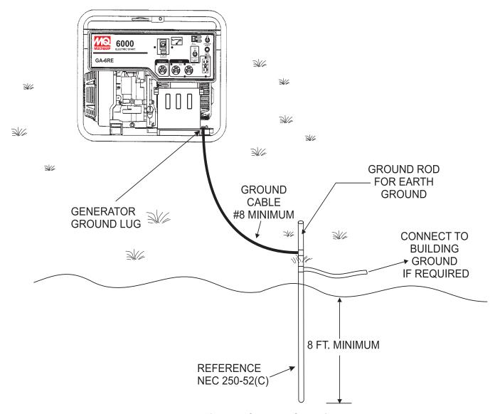
Figure 5. Generator Grounding
