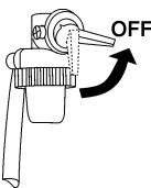
Figure 26. Engine Fuel Valve Lever (OFF Position)
