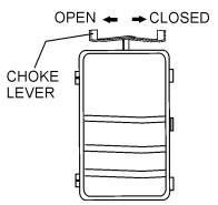
Figure 12. Choke Lever
