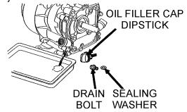
Figure 28. Engine Oil (Draining)
