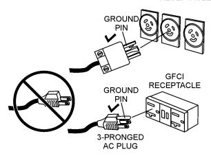
Figure 6. Ground Cables/Plugs
