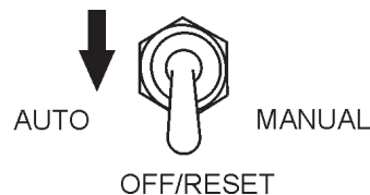
Figure 56. MPEC Control Switch (Off/Reset)
