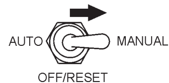
Figure 42. MPEC Control Switch (Manual Position)
