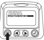
19. Touch the "Menu Button" to exit the Main menu and return to the engine parameter display.
