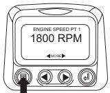
6. Touch the "Menu Button" to exit the Main menu and return to the engine parameter display.
