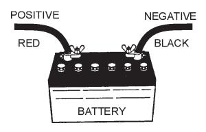
Figure 37. Battery Connections
