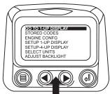
3. Once the "Adjust Contrast" menu item has been highlighted touch the "Enter Button" to activate the "Adjust Contrast" function.
