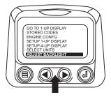
3. Once the "Adjust Backlight" menu item has been highlighted touch the "Enter Button" to activate the "Adjust Backlight" function.
