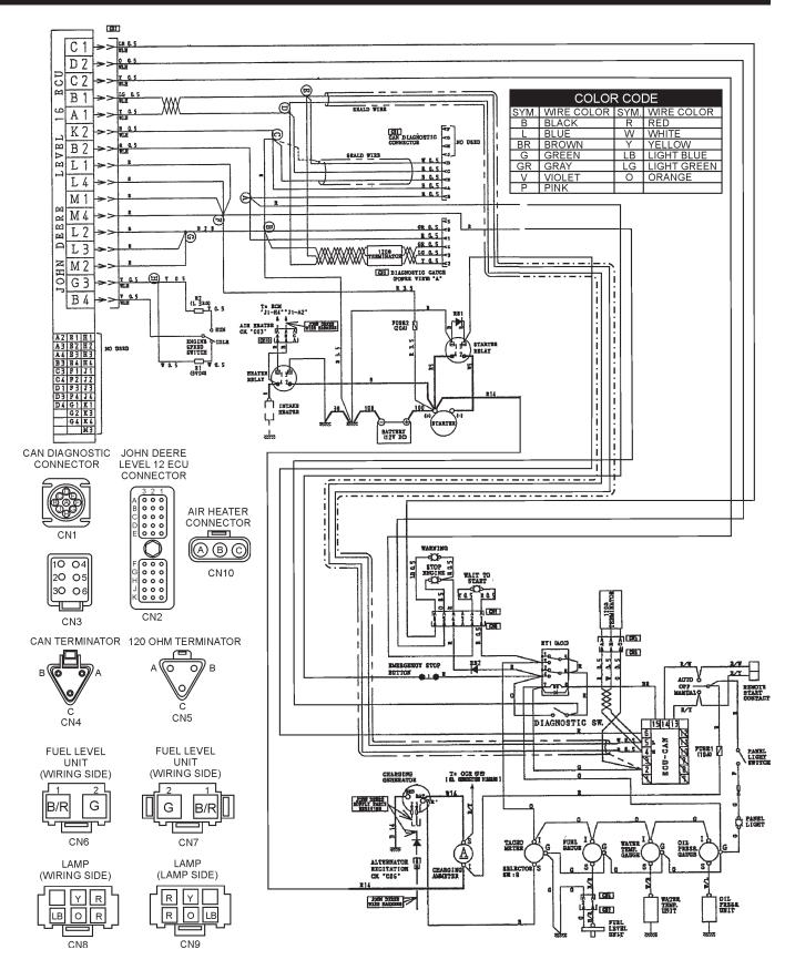
Figure 64. Engine Wiring Diagram
