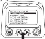
3. Once the "Stored Fault Codes" menu item has been highlighted touch the "Enter Button" to view the "Stored Fault Codes" (when applicable, consult engine or transmission manufacturer for SAE J1939 supported parameters).
