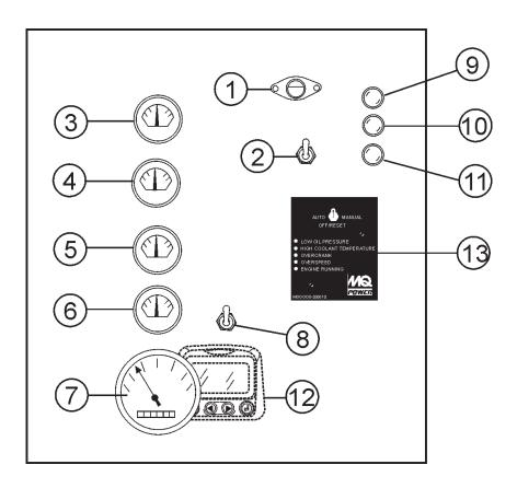
Figure 8. Engine Operating Panel
