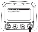
5. The "Use Defaults" screen will be displayed during the resetting period then will automatically return to the "Setup 4- Up Display" menu.
