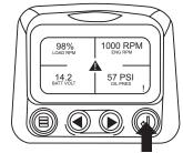
6. Touching the "Enter Button" once again will hide the fault and return the screen to the single or four parameter display.
