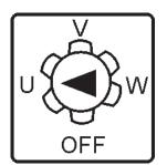
Figure 19. AC Ammeter Change-Over Switch
