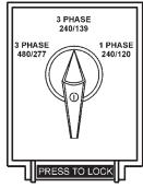
Figure 22. Voltage Selector Switch 240/139V Three-Phase Position
