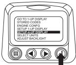
4. Touch the "Enter Button" to activate the "Use Defaults" function. This action will reset the unit to the factory default.
