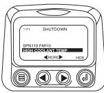
3. To acknowledge and "Hide" the fault and return to the single or four parameter display touch the "Enter Button".
