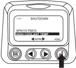
6. The Single or Four parameter screen will display the fault icon until the fault condition is corrected. NOTE: Ignoring active fault codes could result in severe engine damage.
