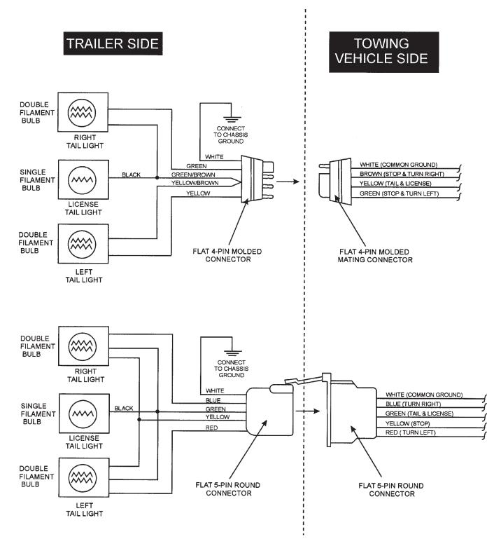
Figure 62. Trailer/Towing Vehicle Wiring Diagram
