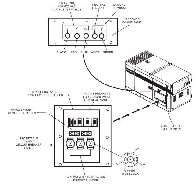
Figure 9. Output Terminal Panel
