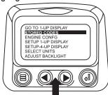
3. Once the "Stored Fault Codes" menu item has been highlighted touch the "Enter Button" to view the "Stored Fault Codes" (when applicable, consult engine or transmission manufacturer for SAE J1939 supported parameters).
