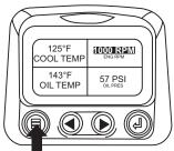
15. Touch the "Menu Button" to exit the Main menu and return to the engine parameter display.
