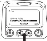
4. To acknowledge and "Hide" the fault and return to the single or four parameter display touch the "Enter Button".
