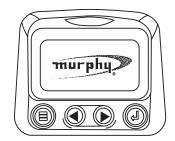
2. The "Wait to Start" message will be displayed for engines with a pre-startup sequence. Once the "Wait to Start" message is no longer displayed the operator may start the engine. Note: Displays only when SAE J1939 message is supported by engine manufacturer.
