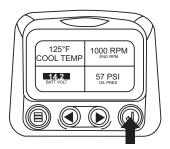
9. The parameter that is highlighted is the selected parameter for the screen. Use the "Arrow Buttons" to highlight the new parameter to be placed in the quadrant selected in the previous screen.
