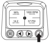
5. Touching the "Enter Button" once again will hide the fault and return the screen to the single or four parameter display.
