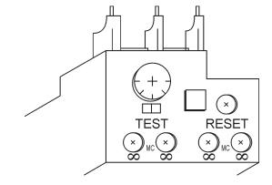
Figure 15. Over Current Relay
