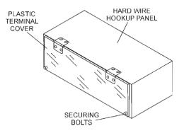
Figure 13. Plastic Face Plate (Output Terminal Lugs)
