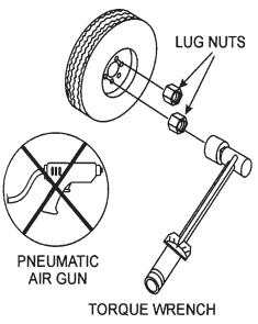
Figure 61. Wheel Lug Nuts Tightening Sequence
