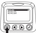
7. Touch the "Menu Button" to exit the Main menu and return to the engine parameter display.
