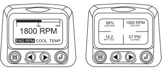
2. When the diagnostic display receives a severe fault code from an engine control unit the single or four parameter screen will be replaced with the "Shutdown" message.
