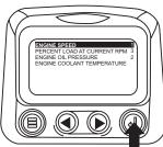
12. Use the "Arrow Button" to scroll and highlight the desired parameter that has not been selected for display.
