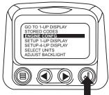
4. Use the "Arrow Buttons" to scroll through the engine configuration data.
