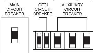
Figure 39. Main, Aux. and GFCI Circuit Breakers (OFF)
