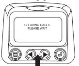
8. When the gage data has cleared, the display automatically returns to the "Utilities" menu. Scroll to "Software Version". Touch "Select" to view the software version currently in the diagnostic display.
