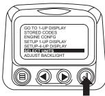
4. Use the arrows to highlight the desired units. "English" for imperial units i.e. PSI,"F or Metric kPa, Metric Bar for IS units i.e. kPa, Bar, "C.
