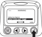
7. The Single or Four parameter screen will display the fault icon until the fault condition is corrected. NOTE: Ignoring active fault codes could result in severe engine damage.
