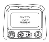
3. Once the engine has started the single engine parameter is displayed.
