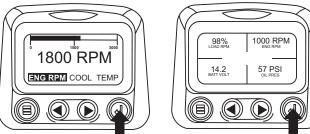
2. The main menu will pop up on the display. Use the "Arrow Buttons" to scroll through the menu until the "Adjust Backlight" is highlighted.
