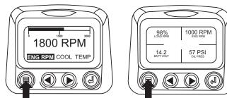
2. The main menu will pop up on the display. Use the "Arrow Buttons" to scroll through the menu until the "Setup 4-Up Display" is highlighted.
