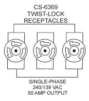
Figure 11. 240/139V Twist-Lock Auxiliary Receptacles Each auxilliary receptacle is protected by a 50 amp circuit breaker. These breakers are located directly above the GFCI receptacles. Remember the load output (current) on all three receptacles is dependent on the load requirements of the *Output Terminal Lugs*.
