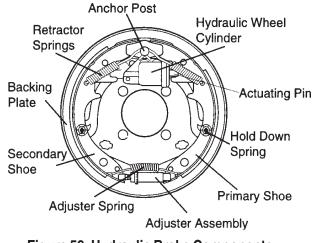
Figure 59. Hydraulic Brake Components
