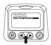
16. Touching the "Enter Button" toggles the "Automatic Scan" function on.
