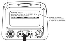
13. Touch the "Enter Button" to select the highlighted parameter for inclusion in the Single Engine Parameter Display.
