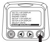
4. Use the "Arrow Buttons" to select the desired backlight intensity.
