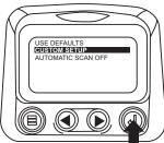
10. Use the "Arrow Buttons" to scroll to and highlight a selected parameter (parameter with a # symbol to right of it).
