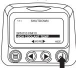
4. The display will return to the single or four parameter display, but the display will contain the "Shut Down" icon. Touching the "Enter Button" will redisplay the hidden fault.
