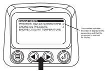
11. Touch the "Enter Button" to deselect the selected parameter removing it from the list of parameters being displayed on the 1-up display.
