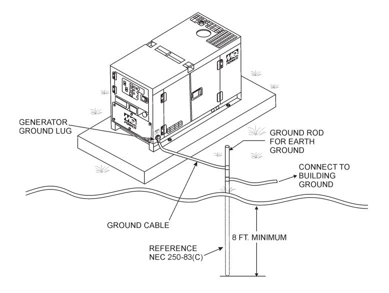
Figure 4. Typical Generator Grounding Application
