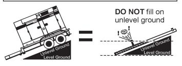
Figure 32. Only Fill on Level Ground
