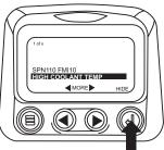
5. The display will return to the single or four parameter display but the display will contain the "Active Fault" warning icon. Touching the "Enter Button" will redisplay the hidden fault.
