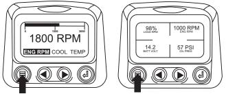
2. The main menu will pop up on the display. Use the "Arrow Buttons" to scroll through the menu until "Adjust Contrast" is highlighted.
