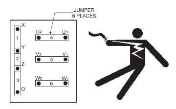
Figure 16. Voltage Change-Over Board
