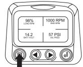
2. The main menu will pop up on the display. Use the arrow buttons to scroll through the menu until the "Select Units" is highlighted.
