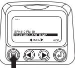
6. Touch the "Menu Button" to exit the Main menu and return to the engine parameter display.
