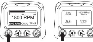
2. The main menu will pop up on the display. Use the "Arrow Buttons" to scroll through the menu until the "Setup 1-up Display" is highlighted.
