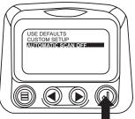
18. Once the "Use Defaults", "Custom Setup" and "Automatic Scan" functions have been set touch the "Menu Button" to return to the main menu.
