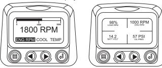
2. The PVA Series of auxiliary gages can be attached to the PowerView. These auxiliary gages communicate with the Modbus master PowerView via a daisy-chained RS-485 port. If at any time during system initialization or normal operation an auxiliary gage should fail, the single or four parameter screen will be replaced with the "MLink Gage Fault" message.
