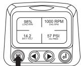
2. When the PowerView receives a fault code from an engine control unit the single or four parameter screen will be replaced with the "Active Fault Codes" message.
