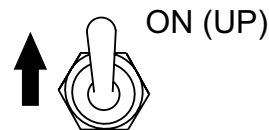
Figure 22. Fuel Priming Switch (ON)
