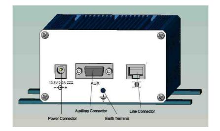
The transmitter requires 13.8VDC at about 2.1A. The DC input to the transmitter is via a 2.1mm connector. To fit the locking type connector to the transmitter, push the connector in and turn it until the two locking lugs enter the socket and none of the connector barrel is visible. Then turn the connector a quarter turn clockwise.
