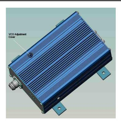
If the VCO control voltage bar is not green, remove the VCO Adjustment Cover from top of transmitter and using a thin non-metallic adjusting tool, adjust CV1 until the control voltage bar is green:
