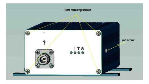
Pull the transmitter circuit board out of the case from the front, with the front panel attached.
