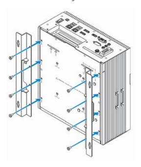
2. Drill four holes in the wall that correspond to the holes in the mounting bracket, then place the system against the wall and align the holes in the mounting brackets with the holes in the wall.
