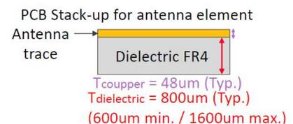
PCB requirement: The dielectric constant of PCB is 4.6, and the impedance boundary is limited to 0.5mm. The thickness of RF trace copper is 48um, and the total thickness of base plate is 1.6mm.
