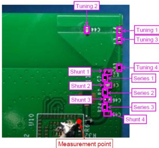
3. Different antenna length and shapes effect radiated emission and each design should be considered a different type:
