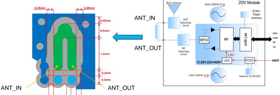
The distance (thickness) between the green pattern and the lower ground is 200 microns.
