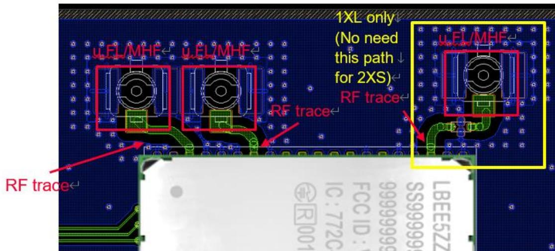
The 50ohm microstrip line needs to be copied when module is installed in the End product.
