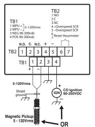
WARNING: In hazardous areas the overspeed relay contact is certified for use ONLY with Murphy non-incendive or intrinsically safe products. In non-hazardous areas overspeed relay contact may be used to switch electromechanical Tattletale® or Magnetic Switches that do not exceed the relay contact rating: 1 A, 30 VDC; 0.3 A, 110 VDC; 0.5 A, 125 VAC. However, the preferred output to switch electromechanical Tattletale® or Magnetic Switches is the N.O. SCR.
