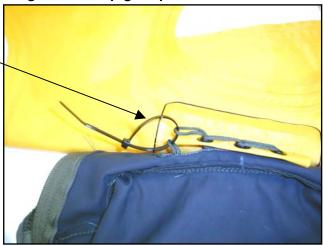
NOTE: Ensure that the plastic self-locking tie ends do not form a sharp point, which may puncture or abrade the inflatable cell.
