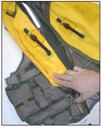
i. Ensuring the zipper does not snag the inflatable cell; ease the slider along the zipper, progressively closing the container over the cell. Tuck the zipper tail inside the opening at the lower edge of the protective container.
