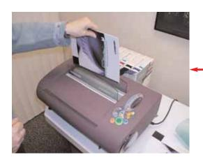
When clamp re-opens, slide book slightly to the left and immediately remove your bound book by lifting it straight up and out of the machine.
