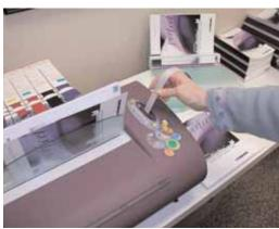
Insert the matching width strip of tape as indicated by the illuminated lamp next to the letter A, B, C, D, E or F in your choice of color, positioning the adhesive coated side of the strip facing the book to be bound. (Glue side up or left, cloth side down or right)
