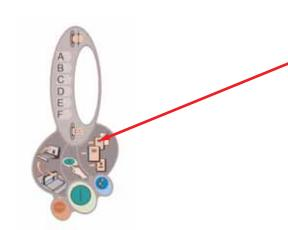
Confirm that the machine has been set for "Editing" mode as indicated by the lamp, if another mode lamp is lit, press the blue button until the correct lamp illuminates. At this time the "insert book" indicator should also be lighted.
