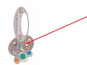
Confirm that the machine has been set for "Normal" binding mode as indicated by the lamp, if another mode lamp is lit, press the blue button until the correct lamp illuminates. At this time the "insert book" indicator should also be lighted.
