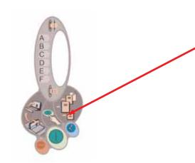
Confirm that the machine has been set for "Pre-Bound" binding mode as indicated by the lamp, if another mode lamp is lit, press the blue button until the correct lamp illuminates. At this time the "insert book" indicator should also be lighted.
