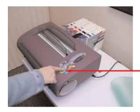
**3.** Press the green Start button to calibrate the AccuBind<sub>Pro.</sub> (Please note that this step is required only when the machine has been powered from off to on or the main cover has been opened)
