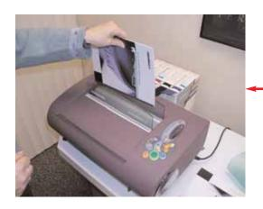
When clamp re-opens, slide book slightly to the left and immediately remove your bound book by lifting it straight up and out of the machine. Do not leave bound book in machine for more than five seconds.
