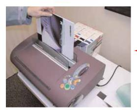
Insert book to be bound (binding edge to the bottom) in the center of the clamp opening at the top of the machine so that it rests evenly on the heating plate below. Slide book fully to the right end. Continue to hold the book and maintain a slight pressure to the right end.
