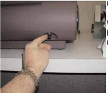
Open the two wing screws. Lift the lid until the stop lever engages.
