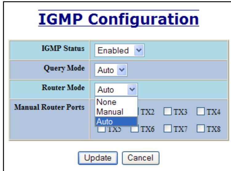
The screenshot shows the 'IGMP Configuration' form. The 'Router Mode' dropdown menu is open, showing options: 'None', 'Manual', and 'Auto'. The 'Manual Router Ports' section contains eight checkboxes labeled TX1 through TX8, all of which are currently unchecked. The 'Update' and 'Cancel' buttons are visible at the bottom.
