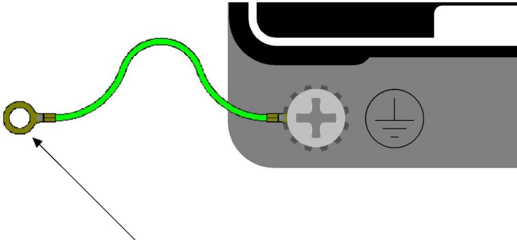
Drain wire with lug connecting switch chassis to known grounding point.
