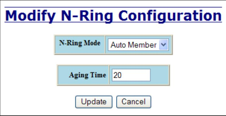
The screenshot shows the 'Modify N-Ring Configuration' interface. It features a title bar with the text 'Modify N-Ring Configuration' in blue. Below the title bar, there are two main configuration sections. The first section is labeled 'N-Ring Mode' and shows 'Auto Member' as the selected value in a dropdown menu. The second section is labeled 'Aging Time' and shows '20' as the value in a text input field. Below these sections, there are two buttons: 'Update' and 'Cancel'.
