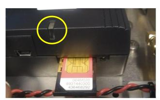
Figure 25: GPRS Modem status LED
