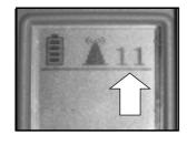
Channel number: When changing the frequency the channel number lights up in the display (HyPro). During operation the choosen channel can be shown by pressing the "FREQUENCY CHANGE" key.
