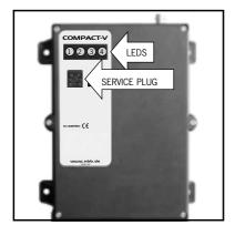
Checking the LED's at the receiver Compact-V:
