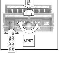
The power supply to the transmitter is activated with the "STOP" key, resp. EMERGENCY STOP switch.
