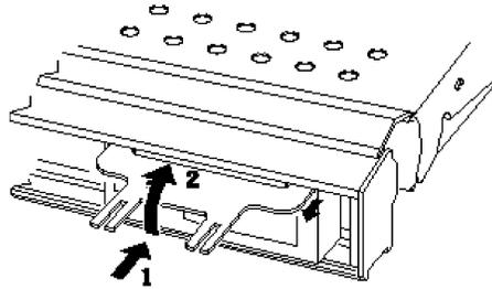
1. Insert the EPL Removal Tool and push it against the rail.
