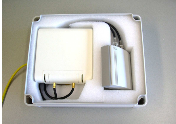
Figure 23. Antenna does not fit into the hole.
