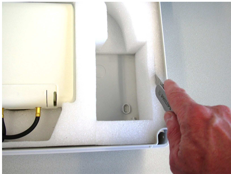
Figure 24. Cutting the foam to allow the antenna to fit into it, in the required position.
