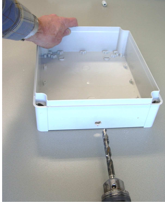
Figure 3. Drilling the hole (12 mm)
