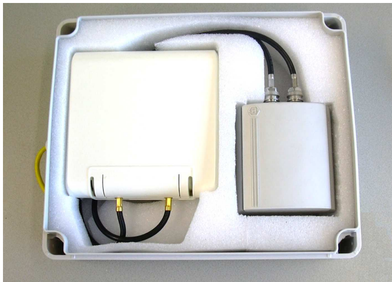
Figure 26. AP300 and directional antenna in their positions.
