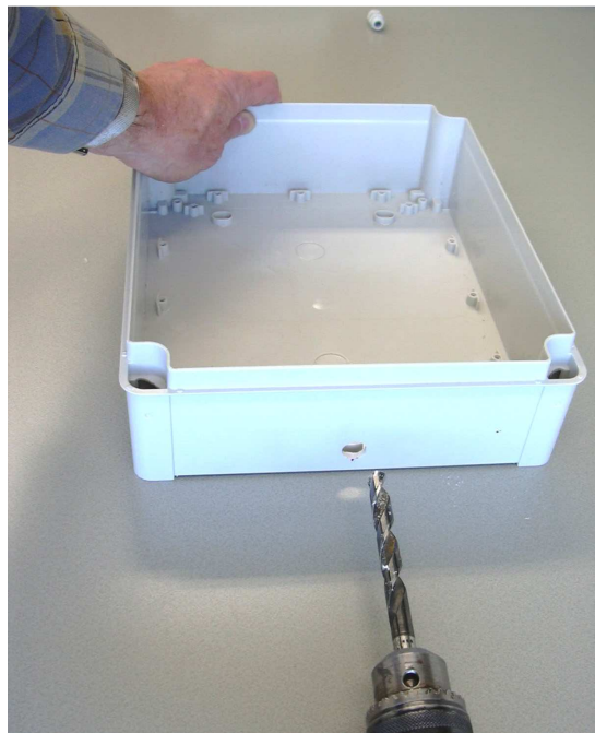
Figure 14. Drilling the hole (12 mm)
