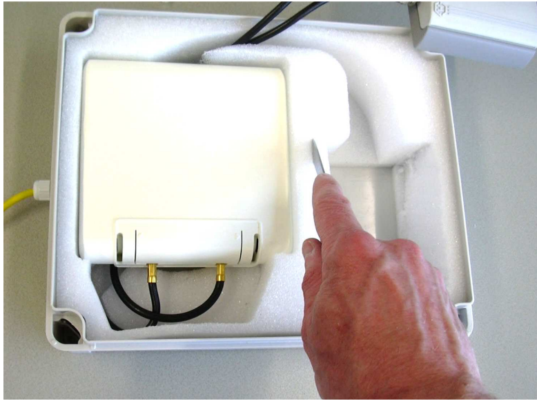
Figure 25. Cutting the foam to allow the antenna to fit into it, in the required position.
