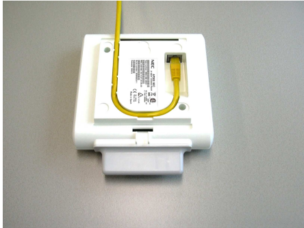
Figure 15. Cable at rear side of the cabinet.
