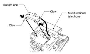
16 Uncover the bottom unit mounted in the Bluetooth<sup>®</sup> cradle (BTC) while holding its knob.
