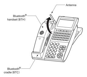
The transformation of the standard handset into a BCH-L(BK) UNIT is complete.
