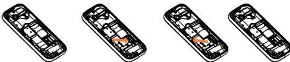
Inserting and removing the SIM card
