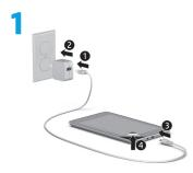
After charging the battery, press and hold the power button for up to 5 seconds until the HP or Compag logo is displayed.
