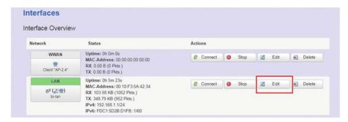
Step 2. Because LAN interface is used for device LAN connection, please make sure that Ethernet Adapter is selected in the "Physical Settings" tab.
