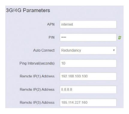
Please select "Redundancy" to enable Wi-Fi and 4G redundant function. You will then need to enter Remote IP address.
