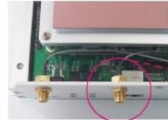
RF cable mounted at the front panel
