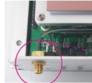
RF cable mounted at the front panel
