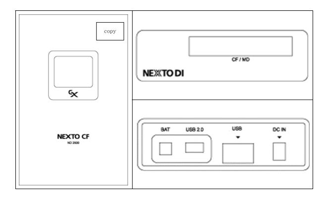
A button and a LCD screen is located on the front panel of Nexto-CF. All the functions of Nexto-CF is controlled by single button. There are 2 ways to press the button. You can either press it once or press it down for more than 2 seconds. On LCD screen the command description is preceded by either "L" of "S" sigh. For "L" sign press down the button for more than 2 seconds and for "S" sign press the button once.
