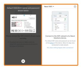
Choose the default SSID of the Vektor and type in the password from the bottom label. Tap on **Join**. Once you are connected, go back to the app.
