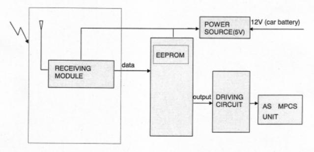
Figure 3.1 block diagram of the receiver
