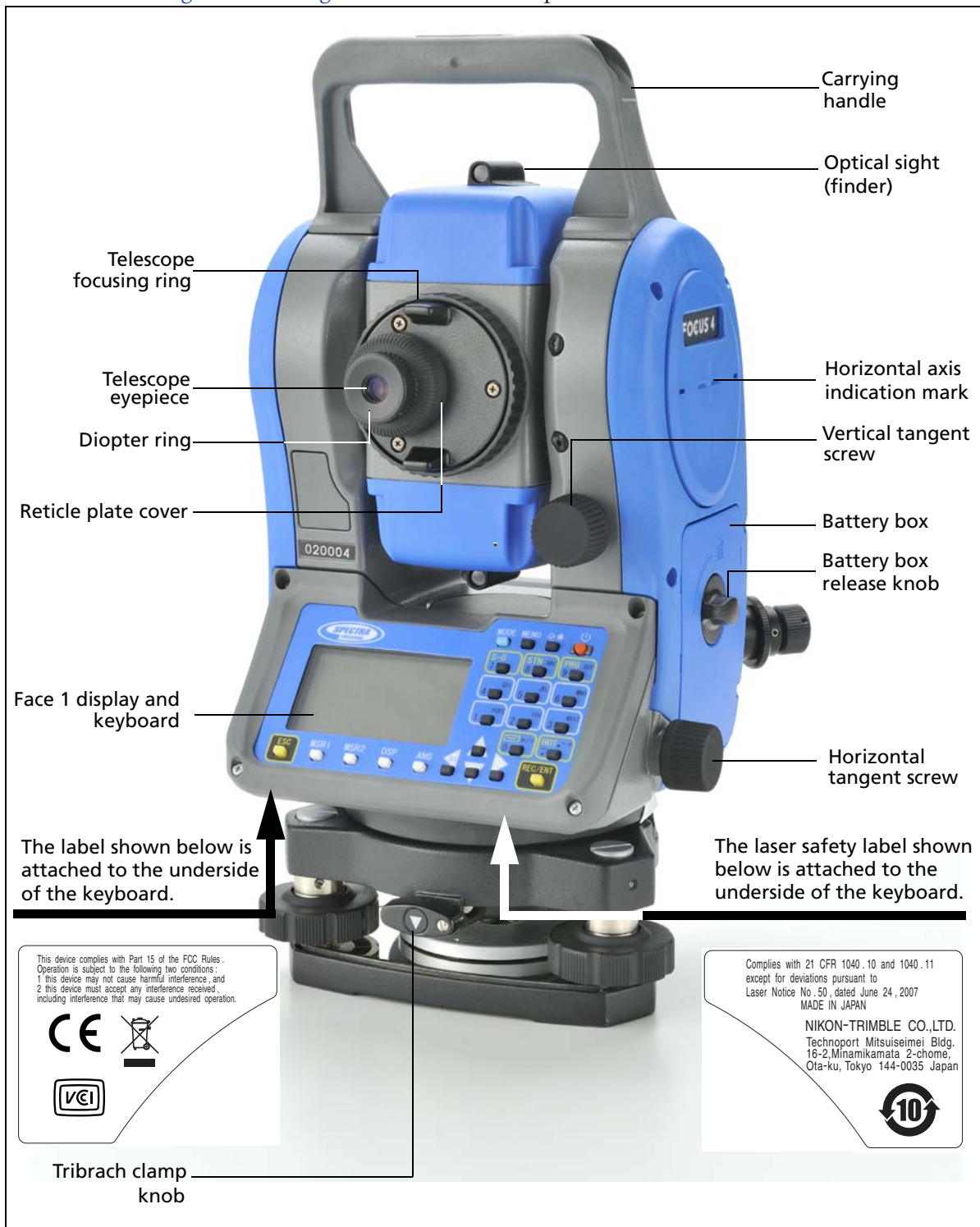
Figure 3.1 Back view of the Focus 4 total station (Face 1)
