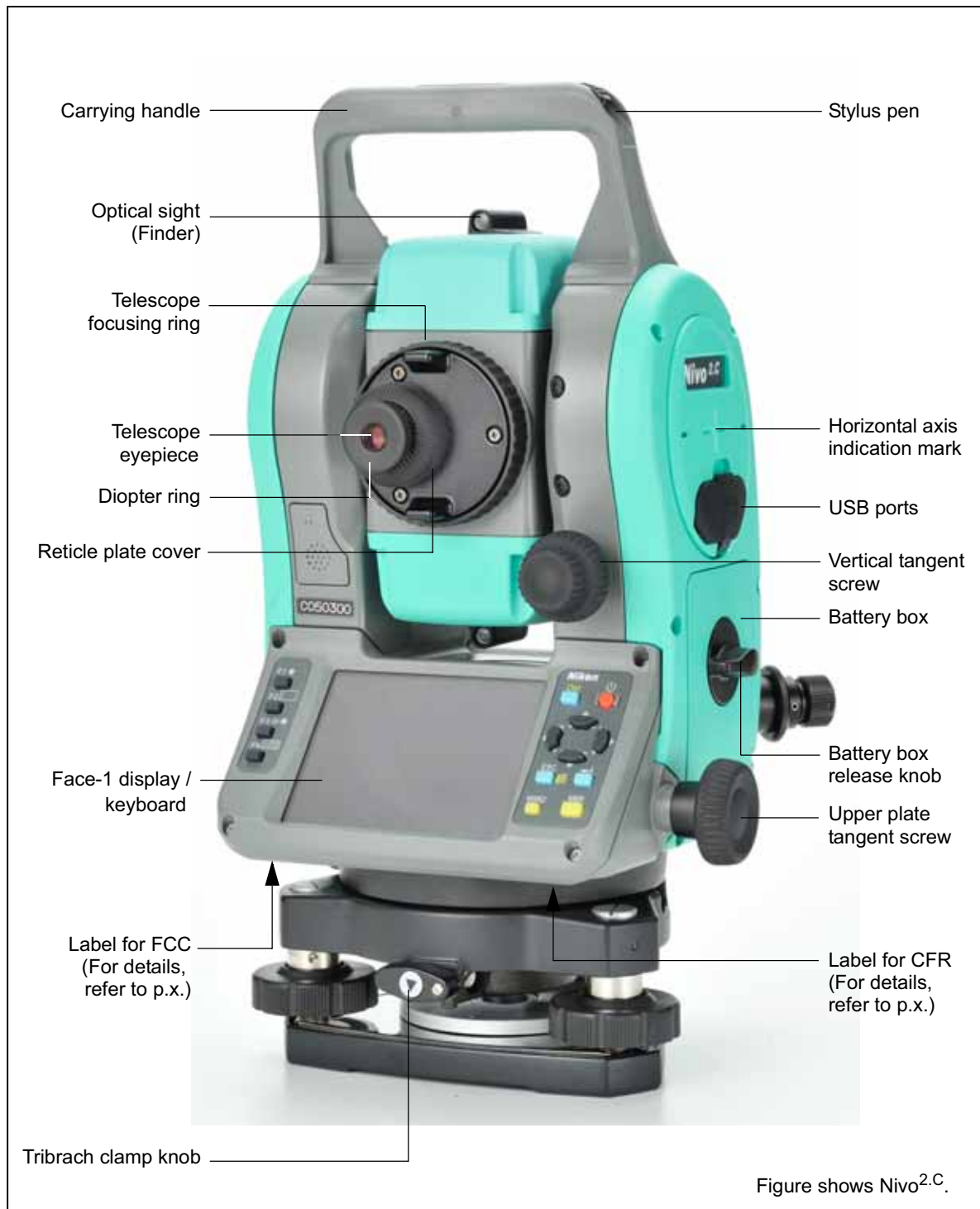
Figure 1.1 Total Station Nivo series – Face-1
