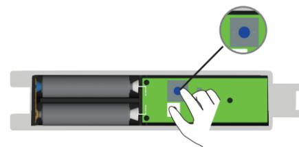
open the outer shell, transmitters have 0 ~ 9 grades switch which used for dial the code for your choose
