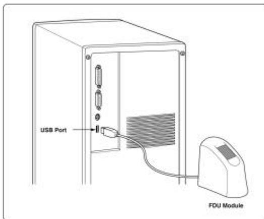
3)The Add New Hardware Wizard will appear when the device is connected. This will search for the new driver for “USB Composite Device”. Click <Next>.
