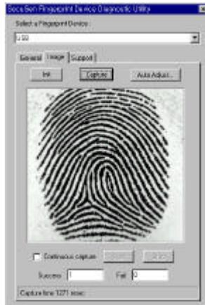
4) If you click <Start> after selecting check box “Continuous Capture”, then fingerprint image appears continuously. At this time, information about the action state of the device appears below.
