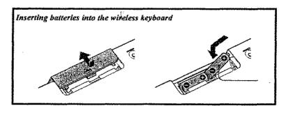
Under normal use, the AA batteries may last up to six months. If your wireless keyboard does not operate properly, the batteries may need to be replaced.
