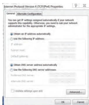
Figure 7: Internet Protocol Version (TCP/IPv4) Properties Dialog Box
