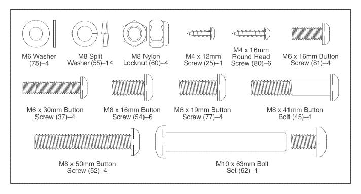
1. Orient the Left Front Stabilizer (15) with the Wheel (17) in the position shown. Attach the Left Front Stabilizer to the left side of the Frame (1) with three M8 x 16mm Button Screws (54) and three M8 Split Washers (55).
