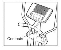
hold the handgrip pulse sensor, with your palms resting against the metal contacts. **Avoid moving your hands or gripping the contacts tightly.**
