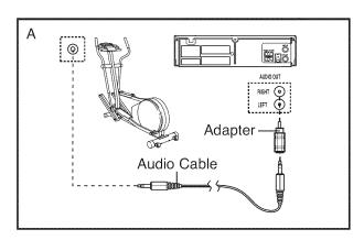
B. Plug one end of the audio cable into the jack beneath the console. Plug the other end of the cable into the adapter. Plug the adapter into an RCA Y-adapter (available at electronics stores).
