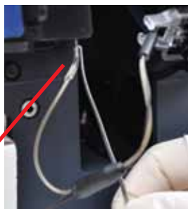
Figure 5.6 Removing Sample Line from Reference Sensor
