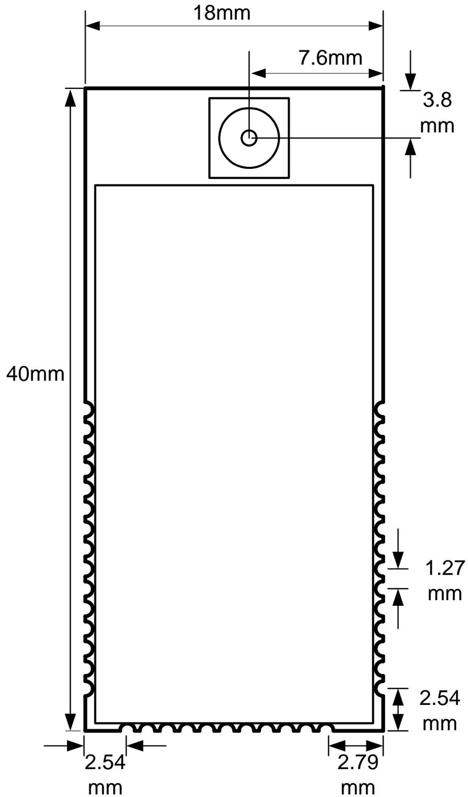
Thickness: 3mm, 10.6mm at SMA connector
