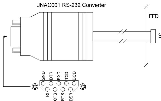
Figure 5-1: JNAC001 RS-232 Converter Connection
