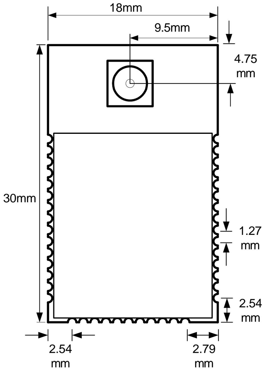
Thickness: 3mm over can, 10.6mm at SMA connector
