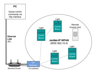
In setting up and using the above demonstration system, the instructions provided in the JN516x-EK001 Evaluation Kit User Guide remain valid with the exception of the references to the JN5168 USB Dongle and the IPv4 address of the Border-Router. In the instructions, the IPv4 address 192.168.11.1 must be replaced with the dynamically assigned (DHCP) IPv4 address of the IoT Gateway.
