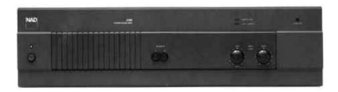
The 2400 has the same features and useful flexibility as the 2100 but produces significantly higher levels of real speaker-driving power. With continuous test tones its output is conservatively rated at IOU watts per channel, while its Power Envelope circuitry produces 370 to 440 watts channel of tone-burst power for music.
