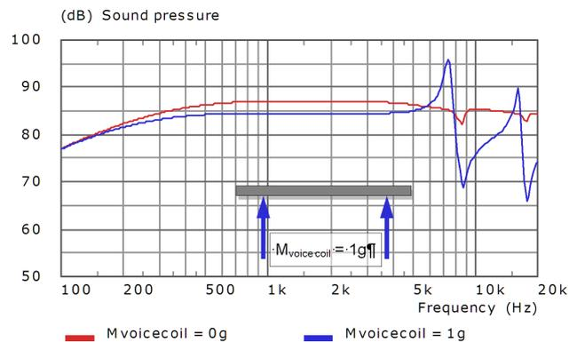
Figure 3. When a motor with finite mass is substituted, the natural balancing of the disk is lost (blue curve)
