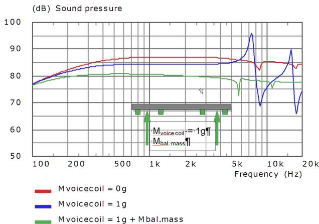
Figure 4. Adding balancing masses restores the behaviour of the free disk (green curve)
