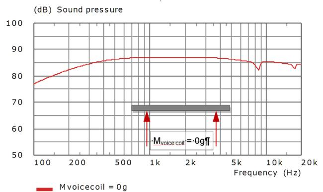
Figure 2. Free disk driven at the first nodal line by an ideal, mass-less force
