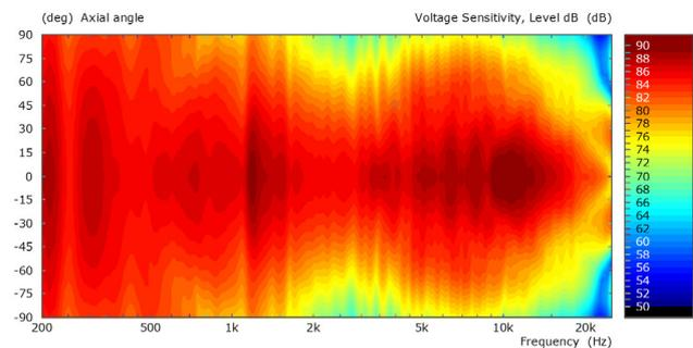
Figure 6. Sound pressure level versus frequency versus angle for the same two-way speaker as Figure 5
