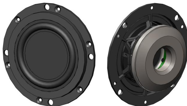
*Front and rear views of the S-800's new 82mm BMR. Key features include a larger, 55mm diameter voice coil and generous rear venting through the neodymium ring magnet*
