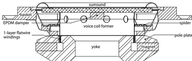
Figure 1. Cross-section of the S-800 Balanced Mode Radiator
