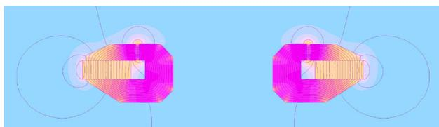
Figure 9. Finite element simulation of flux density within the BMR magnet system
