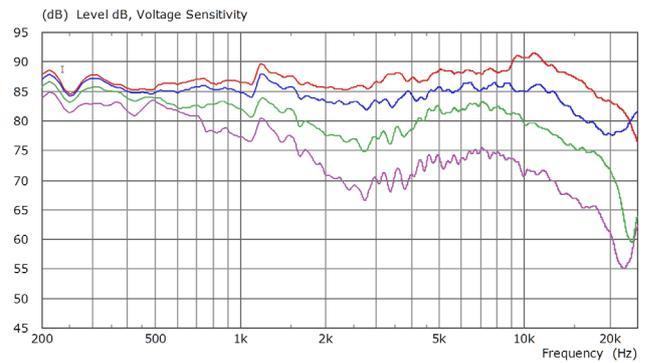
Figure 5. Sound pressure level versus frequency for a two-way speaker at horizontal angles of 0° (on-axis, red), 30° (blue), 60° (green) and 90° (purple)
