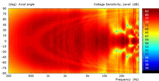
Figure 8. Sound pressure level versus frequency versus angle for the S-800 BMR. Contrast this with Figure 6
