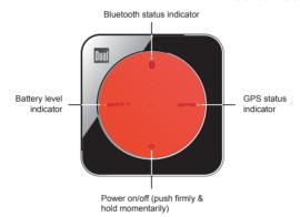
**Power switch**. Firmly press and hold the power icon for a moment to turn the device on or off.
