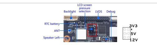
In the above picture, the jumper cap is used to select the screen power supply CON24 from top to bottom, in order:  $3.3V\,/\,5V\,/\,12V$
