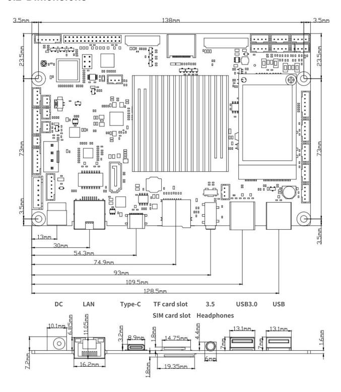
Length: 145mm, Width: 100mm, Front Max. Height: 9mm, Rear Max. Height: 3.5mm. Board thickness: 1.6mm, Screw Hole: Φ3.5mm
