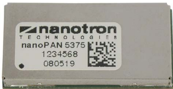
Figure 1: nanoPAN 5375 RF Module – top showing shielding cap
