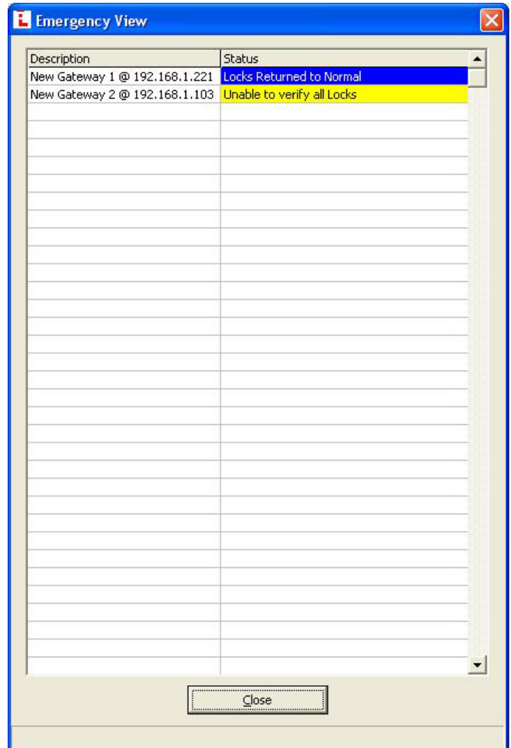
EMERGENCY VIEW SCREEN, DISPLAYING THE STATUS OF LOCKS ASSIGNED TO TWO GATEWAYS
