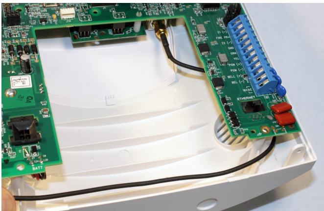
Fig. 6: Route the Antenna Cable to the right of the side "ribs" as shown in this image and in Fig. 7.
