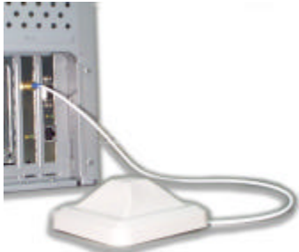
FIGURE 5. CONNECTING THE ADAPTER CARD ANTENNA
