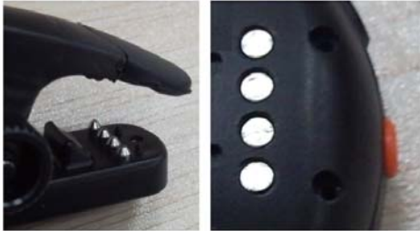
4 contacts at the back of the watch
