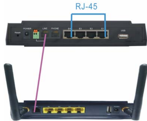
Figure 2.1 NV-720S line ports straight connection
